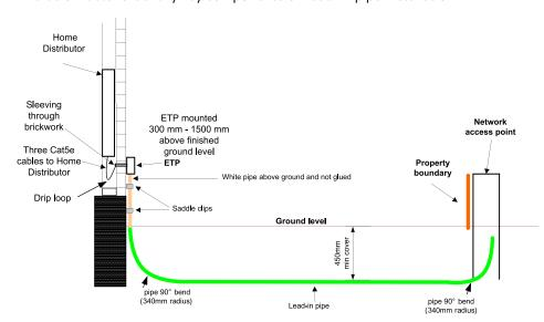
Fig 1. CROSS SECTIONAL VIEW OF A LEAD-IN INSTALLATION
