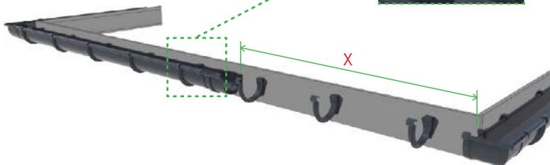
3. Once the solvent is set, insert the length of spouting into the brackets.
