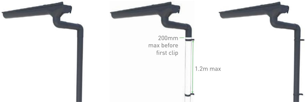
1. Use a level or plumb line to mark the downpipe position against the wall. Dry assemble the downpipe and mark the positioning of the downpipe clips.
