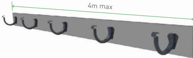
1. Fix the brackets to the fascia with correct spacing from high point to low point (refer to Section 2.1, page 8). Use the recommended fall to the outlet of 5mm per 10 metres.
