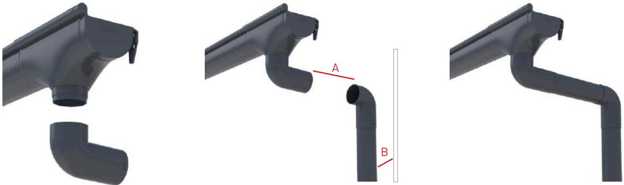
1. Connect the first bend to the expansion outlet. Note: For easy removal of the downpipe assembly for future cleaning and maintenance, screw rather than solvent weld the first bend to the outlet.
