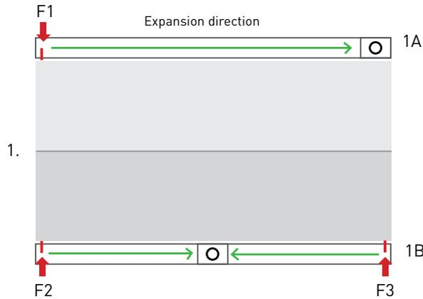
1A. For an expansion outlet positioned at one end of a spouting run, the expansion will be directed from the stop end to the expansion outlet.
