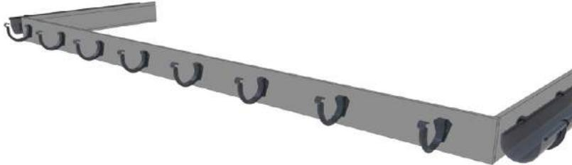
1. Fix the brackets to the fascia with correct spacing from high point to low point (refer to Section 2.1 page 8). Use the recommended fall to the outlet of 5mm per 10 metres.
