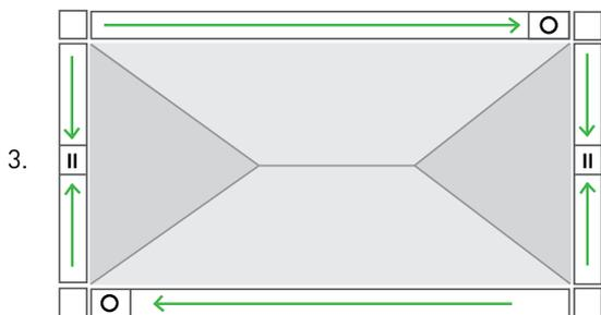
3. For a spouting run exceeding 4 metres between corners without an expansion outlet, an expansion joiner is required. In this instance, the spouting will not require screwing onto the fascia.
