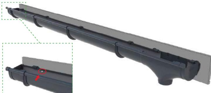
2. Fix the expansion outlet. If terminating the run, refer to Section 2.6 page 8 for stop end installation.
