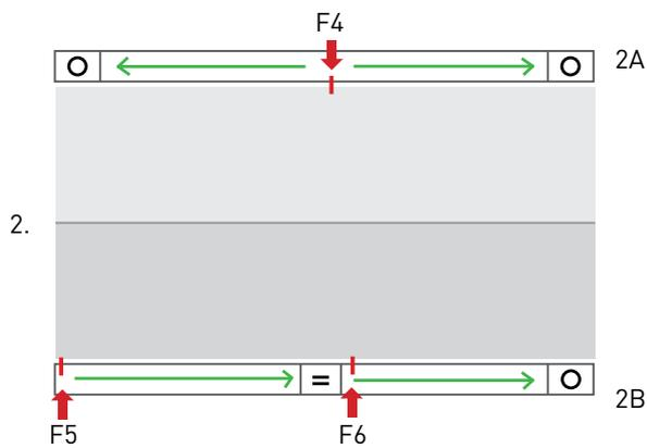
2A. For a long run of spouting with an expansion outlet at each end of the run, fix the spouting in the middle of the run to direct the expansion towards each outlet.
