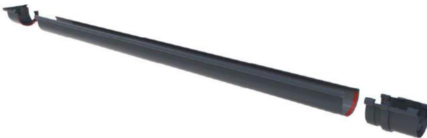
2. At ground level solvent weld the external angle and expansion joiner onto a spouting length. Let this assembly set for at least 10 minutes.
