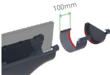
1. Cut 100mm section of spouting and solvent cement the stop end to one end of the spouting.
