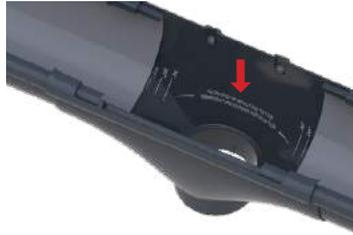
2. Ensure the end of the spouting is aligned with the marking corresponding to the air temperature at the time of installation.
