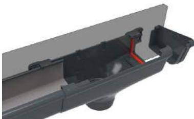
1. Solvent cement both the expansion outlet and the stop end and then connect together.
