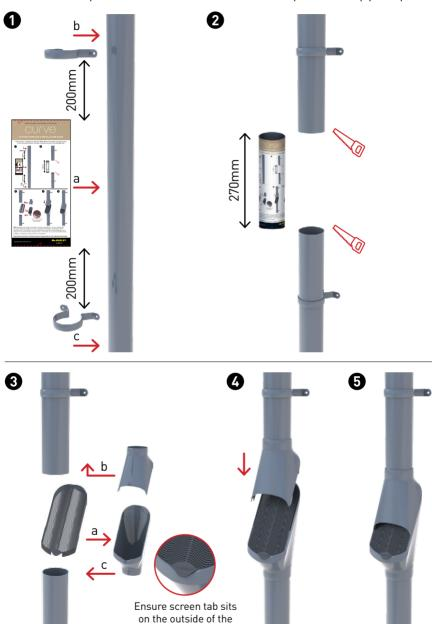
**Note:** Downpipe clip fixings not included - purchase separately to suit your cladding type. Curve should not be installed on metal or rectangular downpipe or on downpipe larger than 80mm OD. If installing Curve in the following scenarios: 65mm uPVC downpipe - extra adaptors are required; Straight downpipe drops - extra bends are recommended; Multistorey buildings - maintenance access needs to be considered.
